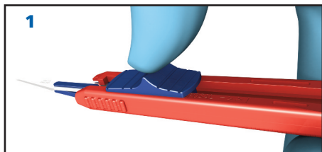
1 Temporary lock in the forward position has been strengthened so that the blade will stay extended even if it encounters a hard surface or bone during use.
